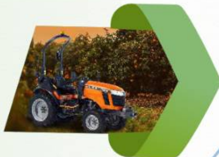
Rollover Protection Structures (ROPS) in one of our tractor models to create a protective zone around the driver when a rollover occurs
